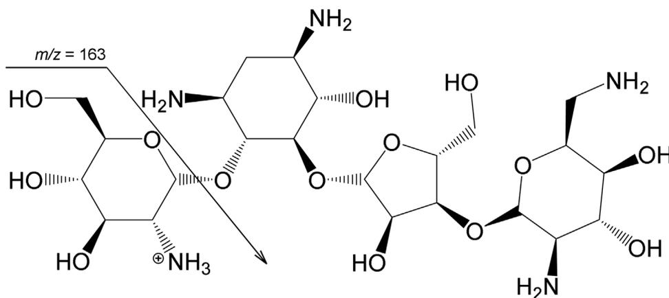
**Fig. 1.** The chemical structure of paromomycin, including the proposed fragmentation pattern and the mass-over-charge ( $m/z$ ) of the monitored product ion. The fragmentation pattern is indicated by an arrow.
