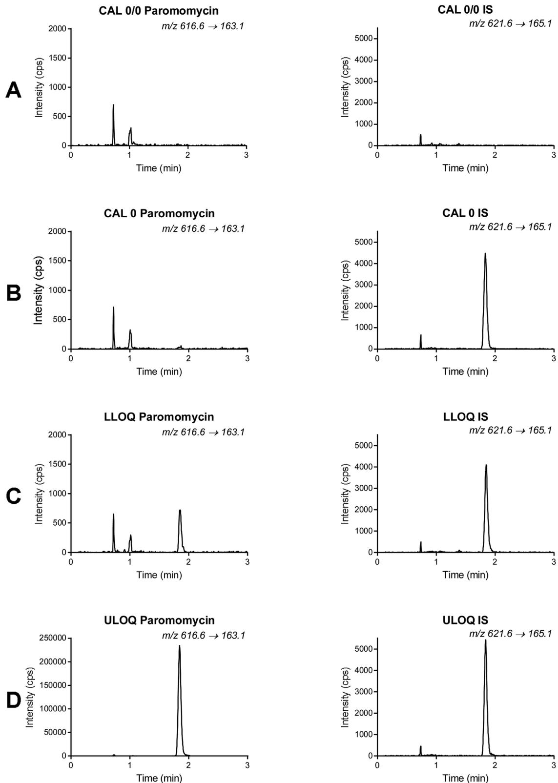
**Fig. 3.** Representative MRM chromatograms of processed human plasma samples. A: double blank (CAL 0/0), B: blank (CAL 0, containing 111 ng/mL internal standard), C: LLOQ (5 ng/mL paromomycin and 111 ng/mL internal standard) and D: ULOQ (1000 ng/mL paromomycin and 111 ng/mL internal standard).
